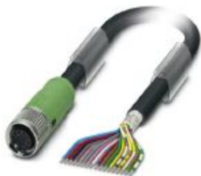
Sensor/actuator cable, 17-position, PUR/PVC, black RAL 9005, shielded, free cable end, on Socket straight M12 SPEEDCON, coding: A, cable length: 1.5 m
