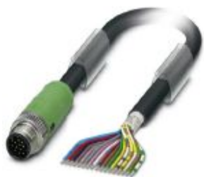
Sensor/actuator cable, 17-position, PUR/PVC, black RAL 9005, shielded, Plug straight M12 SPEEDCON, coding: A, on free cable end, cable length: 5 m
