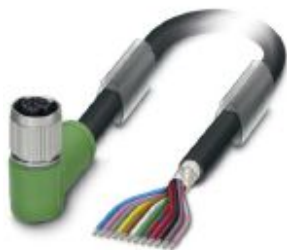
Sensor/actuator cable, 12-position, PUR/PVC, black RAL 9005, shielded, free cable end, on Socket angled M12 SPEEDCON, coding: A, cable length: 1.5 m
