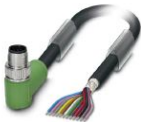
Sensor/actuator cable, 12-position, PUR/PVC, black RAL 9005, shielded, Plug angled M12 SPEEDCON, coding: A, on free cable end, cable length: 10 m
