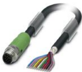
Sensor/actuator cable, 12-position, PUR/PVC, black RAL 9005, shielded, Plug straight M12 SPEEDCON, coding: A, on free cable end, cable length: 1.5 m
