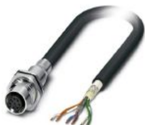
Bus system flush-type socket, VARAN, 6-pos., M12, shielded, rear/screw mounting with M16 thread, with 2 m bus cable
