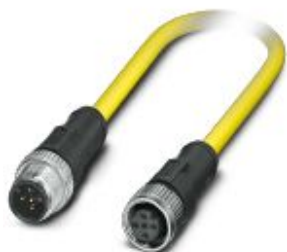
Sensor/actuator cable, 5-position, PVC, yellow, Plug straight M12, coding: A, on Socket straight M12, coding: A, cable length: 20 m
