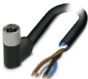
Power cable, 4-position, PVC, black-gray RAL 7021, Socket angled M12, coding: L, on free cable end, cable length: 1.5 m, for direct current up to 16 A/63 V
