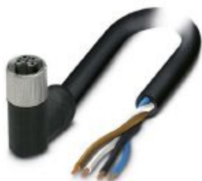
Power cable, 4-position, PUR halogen-free, black-gray RAL 7021, Socket angled M12, coding: L, on free cable end, cable length: 3 m, for direct current up to 16 A/63 V
