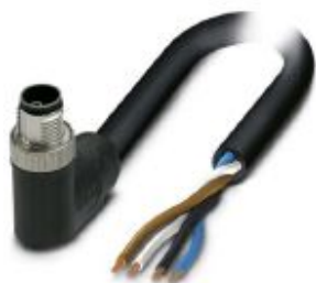
Power cable, 4-position, PVC, black-gray RAL 7021, Plug angled M12, coding: L, on free cable end, cable length: 3 m, For direct current up to 12 A/63 V
