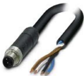
Power cable, 4-position, PVC, black-gray RAL 7021, Plug straight M12, coding: L, on free cable end, cable length: 1.5 m, For direct current up to 12 A/63 V
