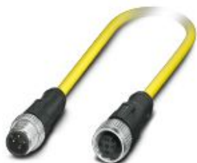
Sensor/actuator cable, 4-position, PVC, yellow, Plug straight M12, coding: A, on Socket straight M12, coding: A, cable length: 3 m
