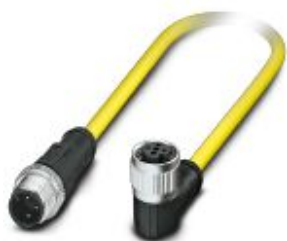
Sensor/actuator cable, 3-position, PVC, yellow, Plug straight M12, coding: A, on Socket angled M12, coding: A, cable length: 5 m
