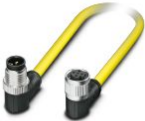
Sensor/actuator cable, 5-position, PVC, yellow, Plug angled M12, coding: A, on Socket angled M12, coding: A, cable length: 0.5 m
