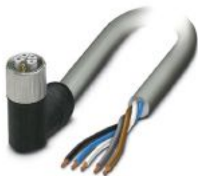
Power cable, 5-position, PVC, gray RAL 7001, Socket angled M12, coding: L, on free cable end, cable length: 5 m, For direct current up to 12 A/63 V
