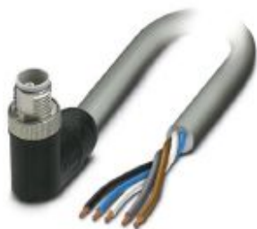
Power cable, 5-position, PVC, gray RAL 7001, Plug angled M12, coding: L, on free cable end, cable length: 5 m, For direct current up to 12 A/63 V
