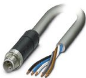
Power cable, 5-position, PVC, gray RAL 7001, Plug straight M12, coding: L, on free cable end, cable length: 5 m, For direct current up to 12 A/63 V
