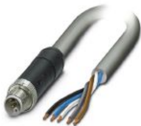
Power cable, 5-position, PVC, gray RAL 7001, Plug straight M12, coding: L, on free cable end, cable length: 1.5 m, For direct current up to 12 A/63 V
