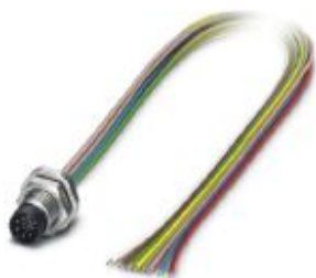
Flush-type connector, 8-position, Plug, straight, M8, Rear mounting, M8 x 1, Individual wires, cable length: 0.5 m, 0.14 mm 2 , PVC litz wire
