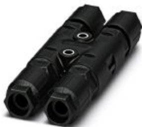
H distributor, QUICKON connection, number of positions: 3+PE, 1 mm 2 ... 2.5 mm 2 , 690 V, 20 A, black, with four QUICKON nuts, cable diameter range: 9 mm ... 14 mm
