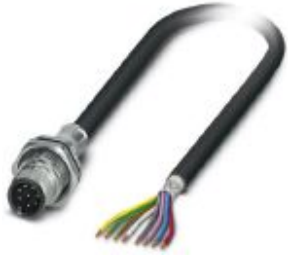
Flush-type plug, shielded, 8-pos., M12, A-coded, rear/screw mounting with M16 thread, with 2 m cable, 8 x 0.25 mm²
