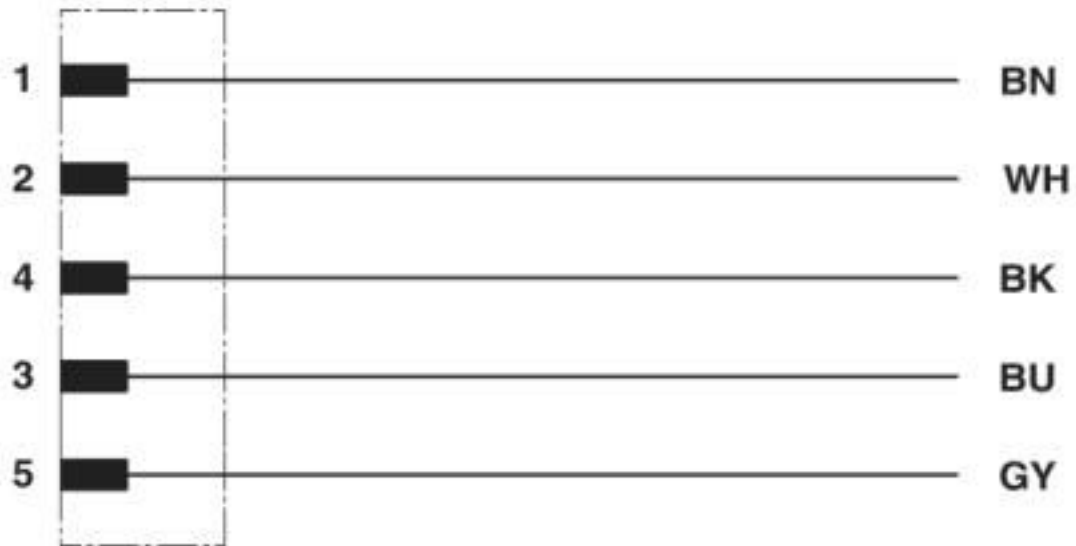
Contact assignment of the M12 plugs
