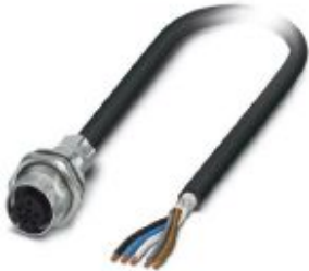
Flush-type socket, shielded, 5-pos., M12, A-coded, rear/screw mounting with M16 thread, with 1 m line, 5 x 0.34 mm²
