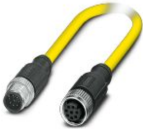
Sensor/actuator cable, 8-position, PVC, yellow, shielded, Plug straight M12, coding: A, on Socket straight M12, coding: A, cable length: 3 m
