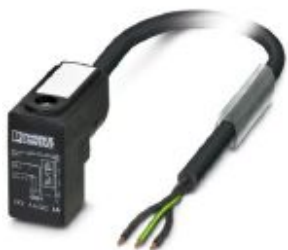
Sensor/actuator cable, 3-position, PVC, black RAL 9005, free cable end, on Valve connector C (8 mm), with 1 LED, connected with Varistor, cable length: 5 m
