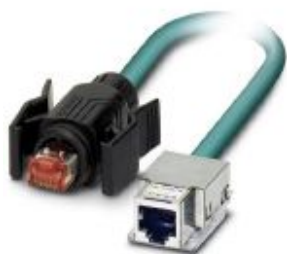
Assembled Ethernet cable, CAT6, shielded, 4-pair, AWG 26 stranded (7-wire), RAL 5021 (water blue), RJ45 socket module/IP20 for Freenet system, 8-pos. on RJ45 plug/IP67, black, line, length 5 m
