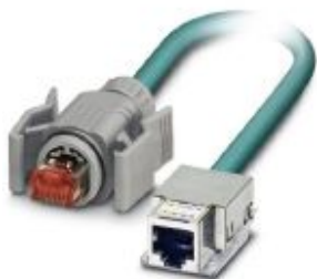
Assembled Ethernet cable, CAT6, shielded, 4-pair, AWG 26 stranded (7-wire), RAL 5021 (water blue), RJ45 socket module/IP20 for Freenet system, 8-pos. on RJ45 plug/IP67, gray, line, length 5 m
