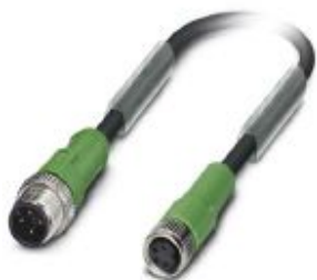
Sensor/actuator cable, 4-position, PVC, black RAL 9005, Plug straight M12, coding: A, on Socket straight M8, cable length: 1.5 m
