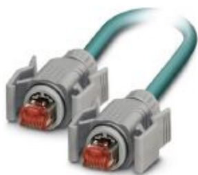
Assembled Ethernet cable, CAT6, shielded, 4-pair, AWG 26 stranded (7-wire), RAL 5021 (water blue), RJ45 plug/IP67, gray on RJ45 plug/IP67, gray, line, length 5 m
