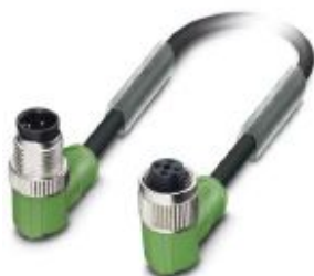
Sensor/actuator cable, 4-position, PVC, black RAL 9005, Plug angled M12, coding: A, on Socket angled M12, coding: A, cable length: 3 m
