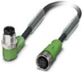
Sensor/actuator cable, 4-position, PVC, black RAL 9005, Plug angled M12, coding: A, on Socket straight M12, coding: A, cable length: 0.6 m
