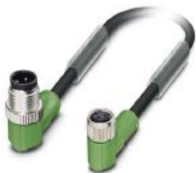
Sensor/actuator cable, 3-position, PVC, black RAL 9005, Plug angled M12, coding: A, on Socket angled M8, cable length: 0.6 m
