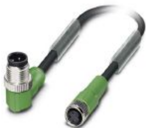
Sensor/actuator cable, 3-position, PVC, black RAL 9005, Plug angled M12, coding: A, on Socket straight M8, cable length: 1.5 m
