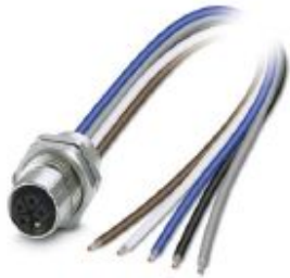
Flush-type connector, Power, 5-position, Socket, M12, L-coded, Rear mounting, M16 x 1.5, Individual wires, cable length: 0.2 m, 2.50 mm 2 , PEX litz wire
