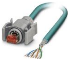
Assembled Ethernet cable, CAT6, shielded, 4-pair, AWG 26 stranded (7-wire), RAL 5021 (water blue), RJ45 plug/IP67, gray on free conductor end, line, length 5 m
