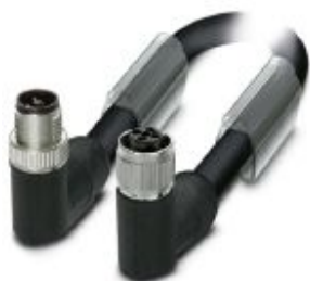
Power cable, 4-position, PUR halogen-free, black-gray RAL 7021, Plug angled M12, coding: T, on Socket angled M12, coding: T, cable length: 2 m, For direct current up to 12 A/63 V
