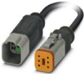
Sensor/actuator cable, 6-position, PUR halogen-free, black-gray RAL 7021, Plug straight DEUTSCH DT04-6P Clip locking, on Socket straight DEUTSCH DT06-6S Clip locking, cable length: 0.3 m
