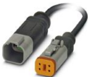
Sensor/actuator cable, 4-position, PUR halogen-free, black-gray RAL 7021, Plug straight DEUTSCH DT04-4P Clip locking, on Socket straight DEUTSCH DT06-4S Clip locking, cable length: 3 m
