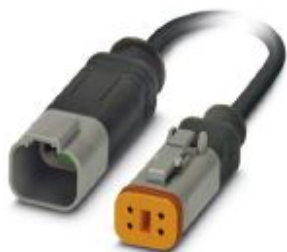
Sensor/actuator cable, 4-position, PUR halogen-free, black-gray RAL 7021, Plug straight DEUTSCH DT04-4P Clip locking, on Socket straight DEUTSCH DT06-4S Clip locking, cable length: 0.6 m
