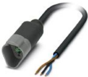
Sensor/actuator cable, 3-position, PUR halogen-free, black-gray RAL 7021, Plug straight DEUTSCH DT04-3P Clip locking, on free cable end, cable length: 10 m
