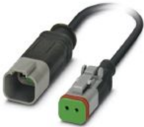
Sensor/actuator cable, 2-position, PUR halogen-free, black-gray RAL 7021, Plug straight DEUTSCH DT04-2P Clip locking, on Socket straight DEUTSCH DT06-2S Clip locking, cable length: 3 m
