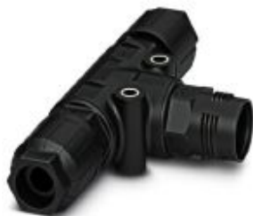
T distributor, QUICKON connection, number of positions: 4+PE, 0.5 mm 2 ... 1.5 mm 2 , 690 V, 17.5 A, black, With two QUICKON nuts, cable diameter range: 10 mm ... 14 mm
