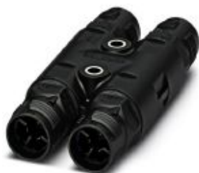
H distributor, QUICKON connection, number of positions: 3+PE, 0.5 mm 2 ... 1.5 mm 2 , 690 V, 17.5 A, black, without QUICKON nut
