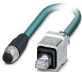
Network cable, Ethernet CAT5 (1 Gbps), 8-position, PUR, Plug straight M12 / IP67, coding: A, on Plug straight RJ45 Push Pull / IP67, cable length: 2 m
