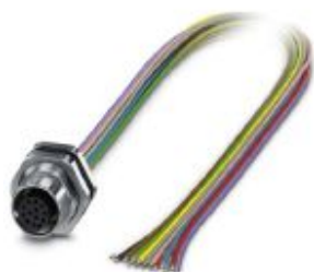
Flush-type connector, Universal, 8-position, Socket, M12, A-coded, Rear mounting, M16 x 1.5, Individual wires, cable length: 0.5 m, 0.25 mm 2 , TPE litz wire
