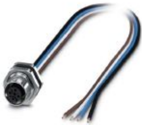
Flush-type connector, Universal, 5-position, Socket, M12, B-coded, Rear mounting, M16 x 1.5, Individual wires, cable length: 0.5 m, 0.34 mm 2 , TPE litz wire
