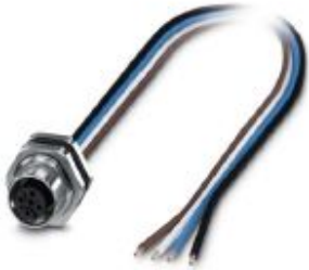
Bus system flat-type plug, 4-position, Socket, M12, D-coded, Rear mounting, M16 x 1.5, Individual wires, cable length: 0.5 m, 0.34 mm², TPE litz wire
