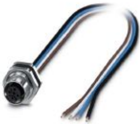
Flush-type connector, Universal, 4-position, Socket, M12, A-coded, Rear mounting, M16 x 1.5, Individual wires, cable length: 0.5 m, 0.34 mm², TPE litz wire
