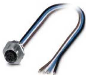
Flush-type connector, Universal, 5-position, Socket, M12, A-coded, Front mounting, M16 x 1.5, Individual wires, cable length: 0.5 m, 0.34 mm², TPE litz wire
