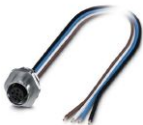
Bus system flat-type plug, PROFINET, 4-position, Socket, M12, D-coded, Front mounting, M16 x 1.5, Individual wires, cable length: 0.5 m, 0.34 mm², TPE litz wire
